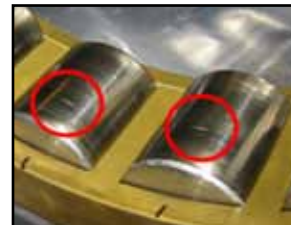
Wear marks on bearing
